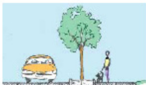
Separated road and trail A buffer strip of vegetation creates a physical separation of automobiles and pedestrians.
