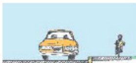
Raised multi-use trail with curb A raised trail bed can provide some protection from vehicles.
